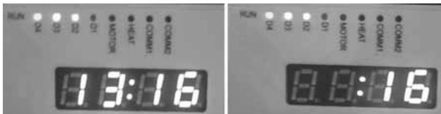
After switching to setting, the time setting will be shown on the indicator as 13:16. The 13 will flicker, press start $\Delta$  or stop  $\nabla$  to adjust the data. Enter next setting by pressing model/setting.
