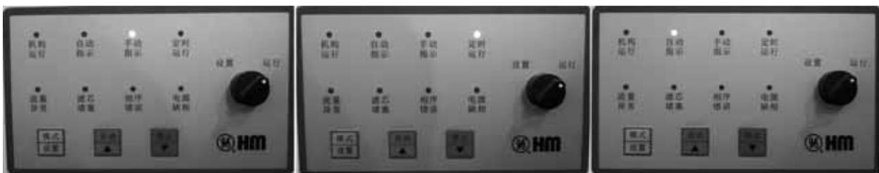
10.2.1 There are three buttons on the controller, namely Mode/setting, on, stop
