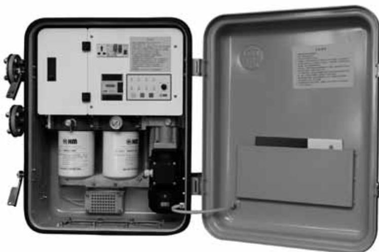
2.3 Type ZXJY-II can be mounted either on the transformer's tank side (referred to as "ON tank type"), or on the ground (referred to as "ground type"). The on tank type is recommended. .
